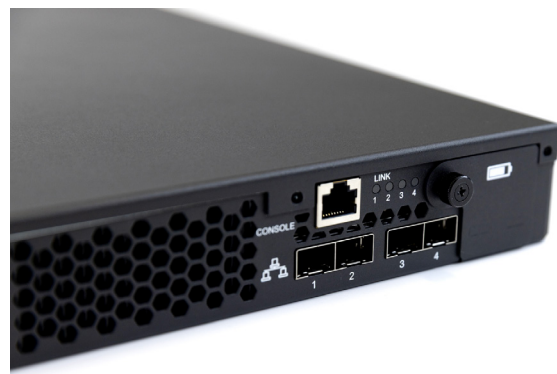
nShield 5c 10G - detail of network interface
