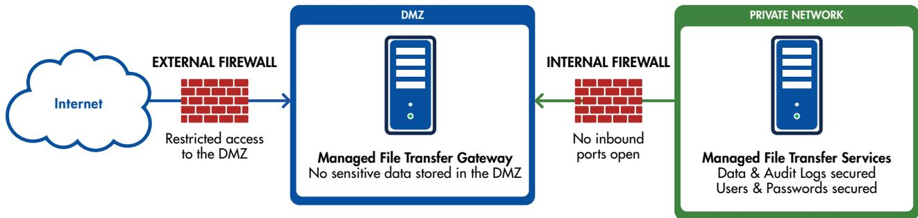
A DMZ gateway functions as both a reverse and forward proxy, keeping sensitive data out of the public-facing DMZ, masking private network addresses, and leaving inbound ports closed to the internal network.
