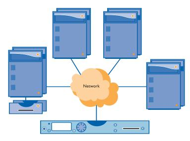
Allows multiple servers to securely access a single HSM
